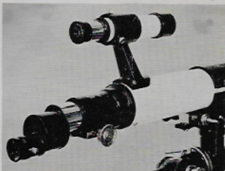
Fig. 8 Erecting Prism and Altazimuth posture
