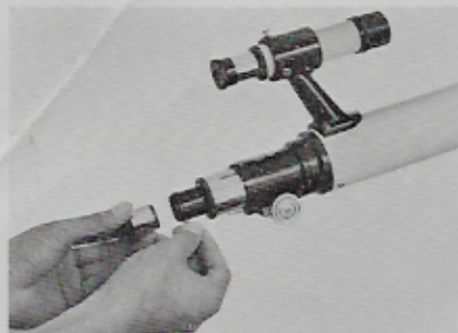
Fig. 4 Inserting the eyepiece into the adapter
