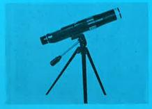
MODEL Z-I: In this beautifully constructed telescope, magnifications of 8X-25X are selected by a recessed knob just forward of the evepiece. The easy-to-operate focussing is by a ring around the telescope body. Object glass diameter 30 mm. Length of telescope 310 mm. Weight 510 gms.
