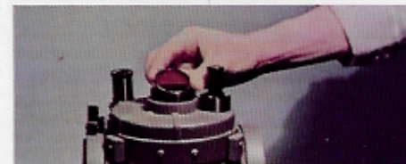
The Celestron accepts Series VI drop-in filters
