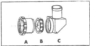
"A" is a special "T"-thread adapter and slip-ring which attaches to the rear threads of your Dynamax. By loosening the slip-ring, you can rotate the entire RFT adapter assembly into convenient observing positions. (Note: this "T" adapter is not the same as our Cassegrain focus adapter you might already own.)
